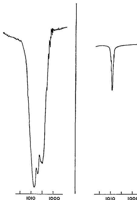
FIG. 6. Infrared spectra of the b_{1u}(\nu_{12}) fundamental of neat C_6H_6 and 1% C_6H_6 in C_6D_6 at 77°K.
